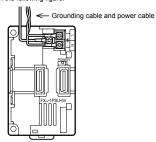
· When connecting an input (only) extension block and an input/output extension block (e.g. FX2N-8ER) to the FX3U-1PSU-5V, supply the power of input circuit for them from the 24V DC service power supply of the nearest preceding main unit or powered extension unit. For details, refer to the following PLC manual.
